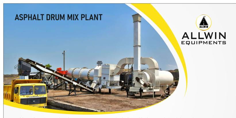
**Cold Feed Hoppers:** Thee / Four Aggregate Bins, Individual variable drives under each bin with precision gates, No Flow Indicator Device, One Bin Vibrator Motor, Highly Accurate Conveying System.
